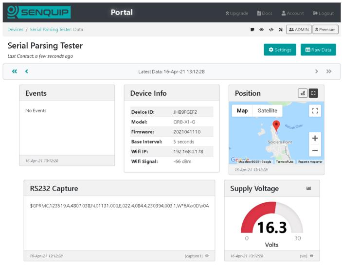
Figure 2 - RMC data being received by an ORB
