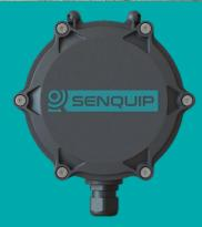
Use the 4-20mA inputs to connect a fuel-compatible 4-20mA level sensor or ultrasonic sensor.
