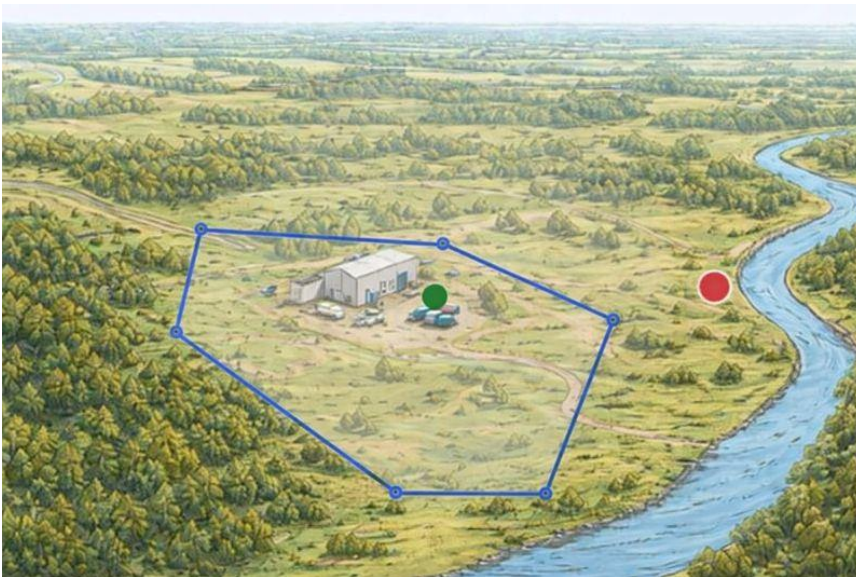
Figure 5 - - Devices Inside and Outside a Polygon Geofence
