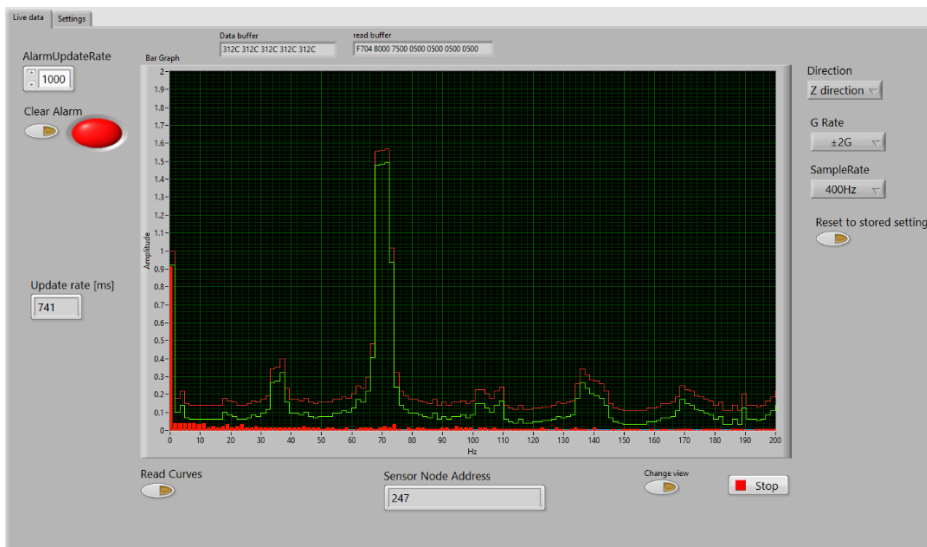
Figure 6 - Supplier Provided Software Showing Live Vibration Data
