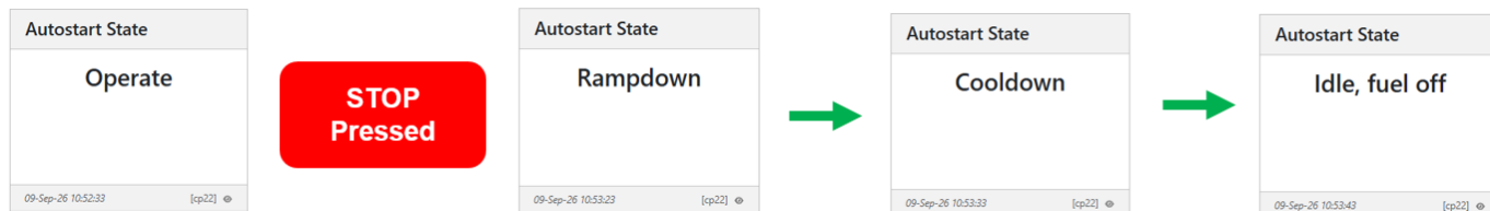
Figure 3 - Sequence of Events Following a Stop Command
